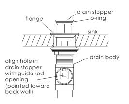
11. Remove rod guide nut and rod ball plastic gasket. Insert horizontal rod into drain body and through hole in drain stopper. Replace rod guide nut with rod ball plastic gasket and tighten it.
