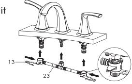
7. Connect the supply lines to the faucet and secure the nuts by adjustable wrench. The hot water supply should go on the left while the cold water supply should go on the right.
