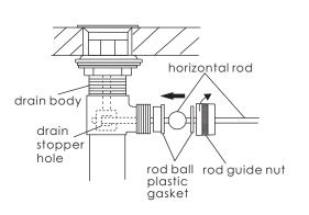
12. Place one end of the spring clip on the end of the horizontal rod. insert the ball rod through a hole on the lift rod strap, then slide the other end of the spring clip over the horizontal rod. See diagram for visual. Hint - Be sure to move the ball rod up and down a few times to make sure the drain stopper opens and closes before going to the next step.
